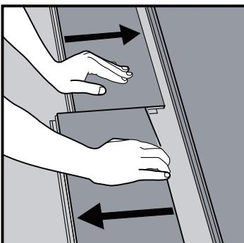
Separate the whole row by lifting it up delicately at an angle.
