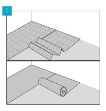
Lay the Arbiton underlay: Multiprotec LVT or Secura LVT Click Smart N perpendicularly to the direction in which panels are laid. The neighbouring ribbons of underlay must be fit tightly and joined by means of an overlap or Arbiton AluTape, without leaving any redundant space.
