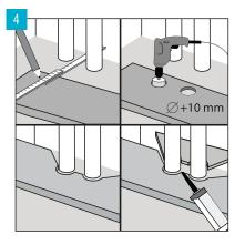
Act similarly in the case of a bigger number heating system pipes. The cut panel elements must be joined with the assembly adhesive for plastic elements.
